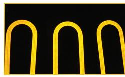
ARI offers high temperature furnace brazing of heaters and sensors to attach directly to the metal parts. Proper heater and sensor attachment allows the parts to remain in contact in a vacuum and not rely on radiant heat transfer. Having that sensing point for feedback to the control system allows excellent repeatability for process control and management.
