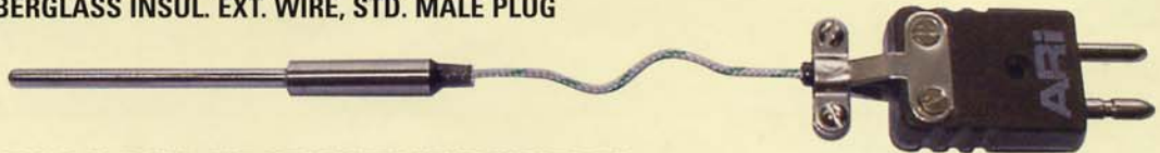
T-99 200°C TRANS. W/FIBERGLASS INSUL. EXT. WIRE WITH ST/ST OVERBRAID
