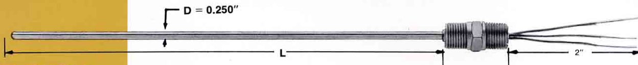
Style PRT-52400.3 with fixed hex nipple Replacement element with 1/2" NPT hex nipple silver brazed to sheath.
